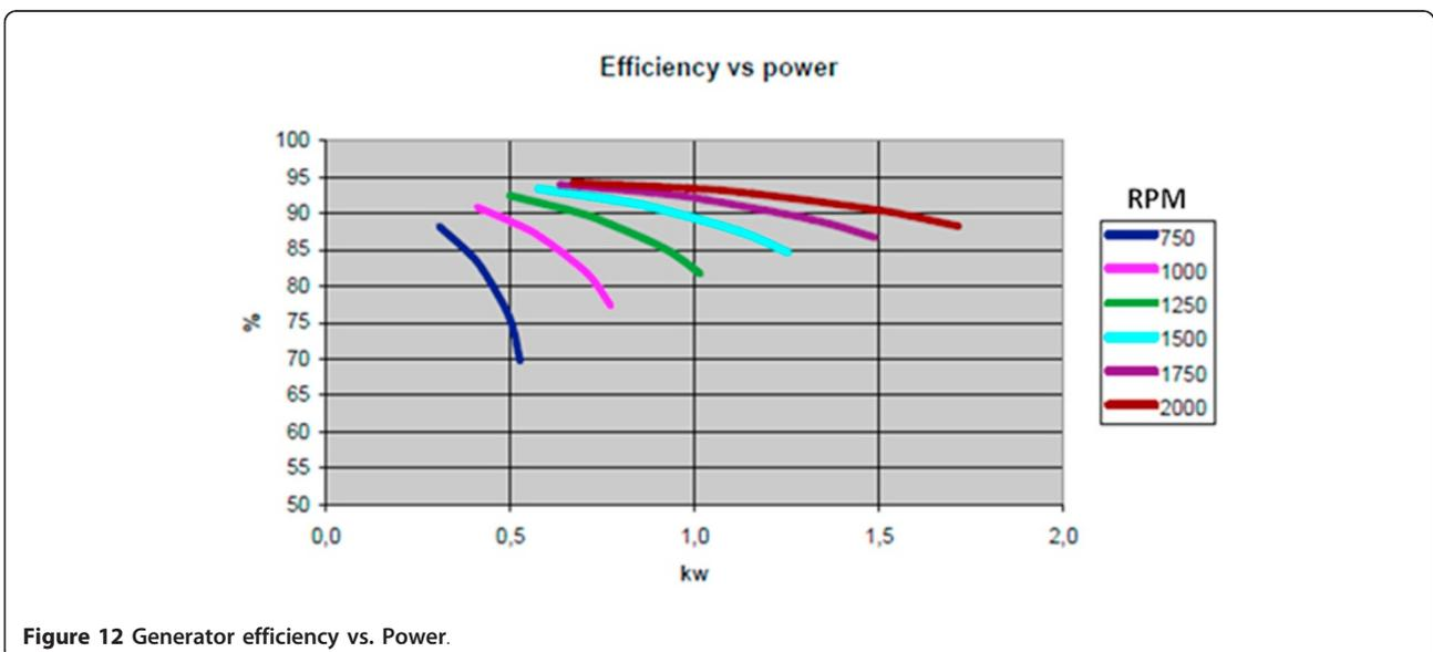
Figure 12 Generator efficiency vs. Power.
