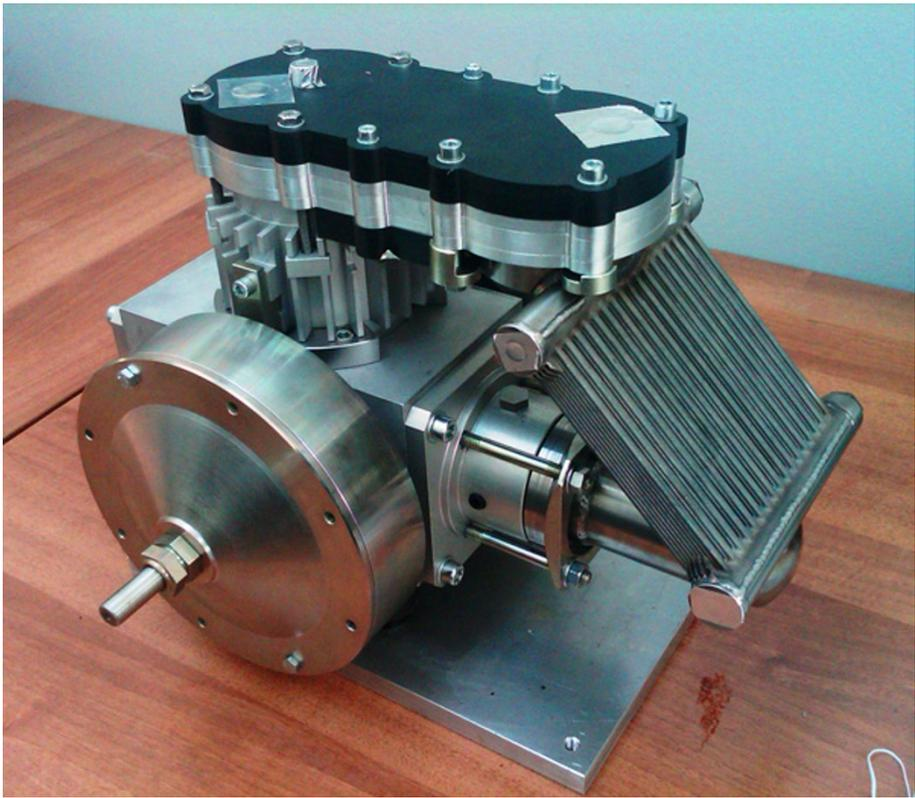
Figure 4 Prototype of the mRT-1k engine under manufacturing and realization in FBK.
